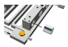
To exchange drill bushings, loosen 1/4-20 set screw until bushing comes out replace and tighten.
