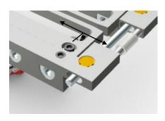
To exchange templates simply loosen screws replace template and tighten screws. Make sure that the template is aligned with respect to the drill bushings and other template, oblong holes in template are provided for this adjustment.
