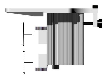
Loosen the bearing screws and adjust bearing up or down accordingly.
