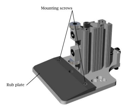
Remove the two rub plate mounting screws, install the trim router to the base (make sure to remove the plastic rub plate that comes with the router before attaching to base). Make sure to align the trim router center to the center of the rub plate hole before tightening. Re-attach the rub plate.
