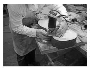
One hand should be holding the binding base handle as shown, the other hand should hold the router base and at the same time rest on the guitar, this will also give control of the router tipping inward. Do not hold router at the top. Then move the router as indicated previously from bout to waist in a smooth motion always keeping both bearings on the side of the guitar and hold the handle perpendicular to the side.
