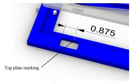
The template has a scale markings in 1/32 increments. This can be used as a reference point when adjusting the dove tail fit.
