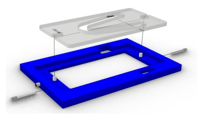
This modification is to allow precise fit and adjustability for the Dove Tail at the neck (tenon) side. The openings for the pins are slotted at both ends so that the template can move up or down in the top plate cavity.
