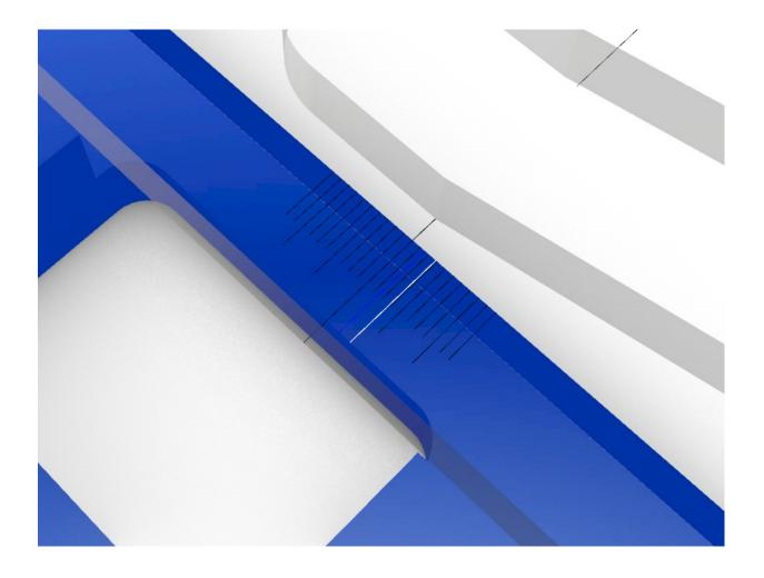
With this modification you should be able to adjust the Dove Tail for fit a either the mortise side and now at the tenon side. The total adjustability is plus 3/8 and minus 3/8
